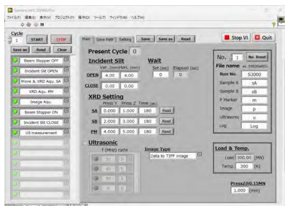
Fig. 2. Newly developed control software for incidence slit and press stage at optical hutch 2, BL04B1.
